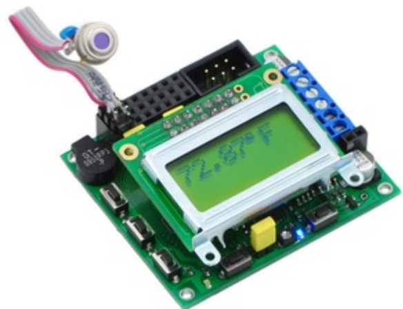
MLX90614 temperature sensor connected to an Orangutan SV-168.
